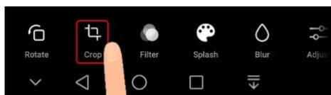
To crop an image, tap the icon, which consists of two interlocking right angles.
